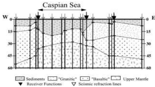
Fig.4. Crust and uppermost mantle cross-section between the Kura basin to the west of the South Caspian basin (y39.5N, 46.0E) and the Turkmenian lowlands and the Kopet dagh mountains to the east (y37.5N, 61.5E): see Fig. 2(b) for location
