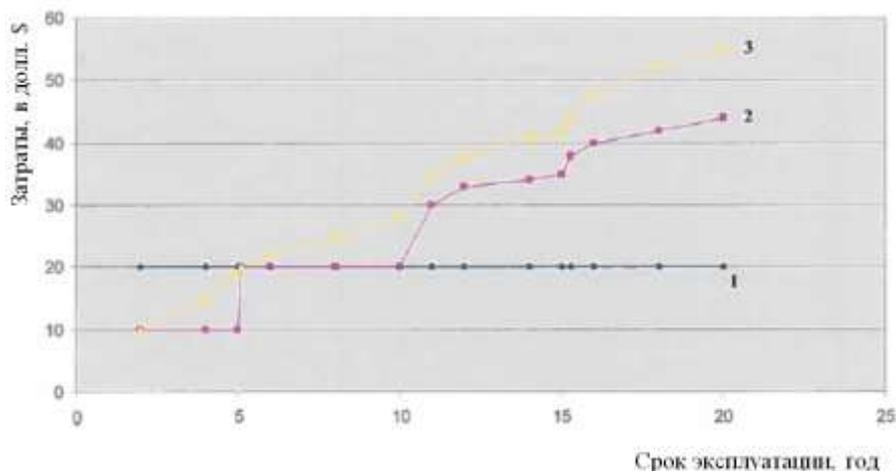
Fig.3. Comparative indicators of the dependence between the cost and service life of basalt plastic and steel pipelines
