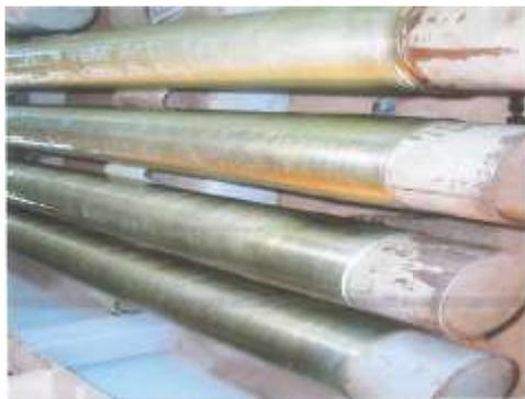
Fig.1. Steel pipes (collector) covered basalt plastic materials
