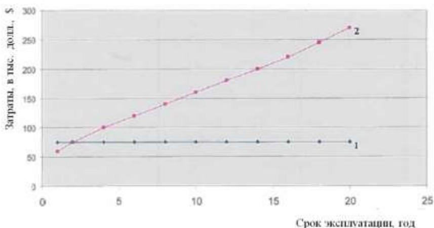
Fig.4. Comparative indicators of the dependence between the cost and service life of basalt plastic and steel pipelines
